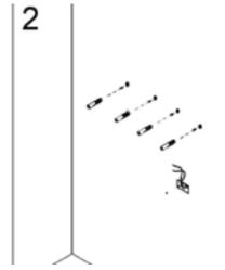
**STEP 2:** Mark on the wall the exact position of mounting screw holes.
