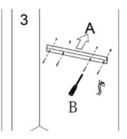
**STEP 3:** Install the back plate on the wall. Make sure it is firmly secured.
